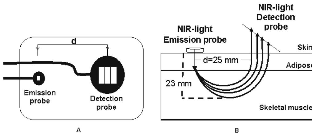
**Fig. 2** **A** Diagram of a distal tip of the NIRS optical cable. **B** With 25 mm spacing ( $d$ ) between emission and detection probes, approx. 95% of the detected optical signal is from 23 mm of tissue penetration
