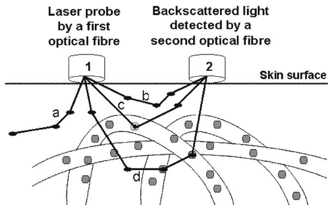
**Fig. 5** Schematic diagram of laser Doppler flowmetry. When the tissue is illuminated by a laser source (1), 93–97% of the light is either absorbed by various structures or undergoes scattering (a, b). The remaining 3–7% is reflected by moving red blood cells (c, d) and returns to the second optical fiber (2). Microvascular perfusion is defined as the product of mean red blood cells (RBC) velocity and mean RBC concentration in the volume of tissue under illumination from the probe
