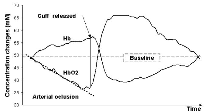
**Fig. 3** Quantitative NIRS measurements during arterial occlusion. After release of the occluding cuff blood volume increases rapidly, resulting in an increase in  $\text{HbO}_2$  and a quick washout of Hb, followed by a hyperemic response. Oxygen consumption is calculated as the rate of decrease in  $\text{HbO}_2$  (dotted line)
