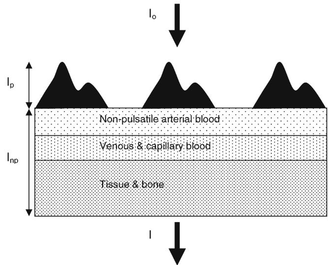
**Fig. 1** The pulsation of arterial blood causes a pulsating volume variation. Peripheral perfusion index (PFI) is calculated as the ratio between the arterial pulsatile component ( $I_p$ ) and the nonpulsatile component ( $I_{np}$ ).  $I_0$  Source light intensity;  $I$  light intensity at the detector
